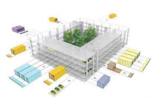
The Kiubo system is extremely simple. High-quality residential units made of wood (modules) are prefabricated in industrial plants. The modules slot into frame-like structures (terminals) and can be configured in numerous ways. This highly flexible slot-in system allows the modules to be inserted, swapped, connected, extended, removed and reinserted elsewhere.
